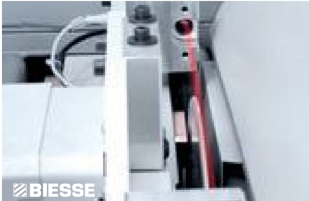
Automatic scoring saw blade alignment system of Selco panel sizing centres.
